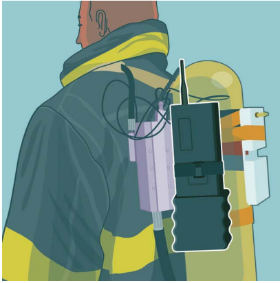
FIGURE 1. A firefighter tests the Precision Personnel Locator system, whose transmitter unit is mounted to the oxygen tank.
