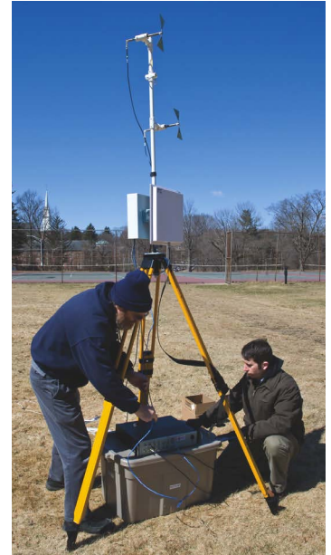
Technician Bob Boisse (left) and graduate student Vincent Amendolare work on a receive station that contains two RF receiving (bowtie) antennas and a wireless Ethernet antenna that receives data from another receive station. The receive unit is inside the bin.
